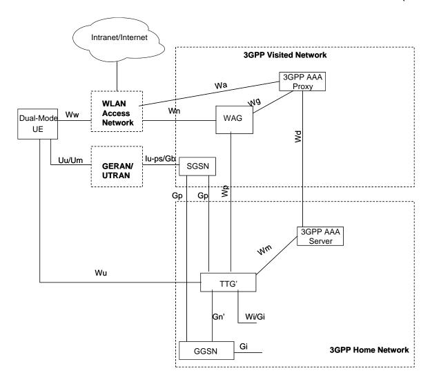
Figure 6.2.2: Roaming Architecture for I-WLAN Mobility
