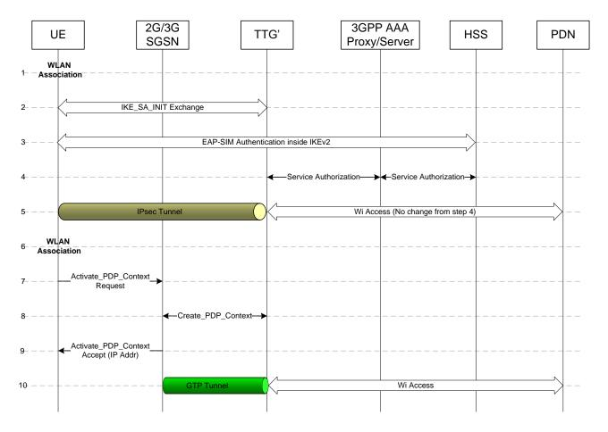
Figure 6.2.5 Handover from pre-SAE 3 GPP to I-WLAN (Wi services)
