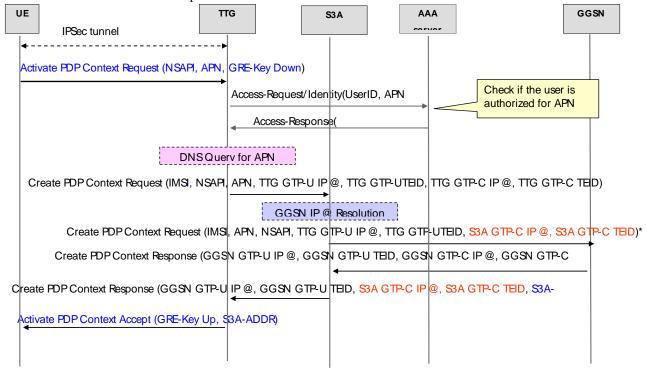
Figure 6.2.11 First PDP context activation on the I-WLAN side
