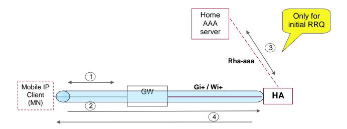
Figure A.2: Use of MIPv4 collocated care-of address mode with Diameter application when no FA is present
