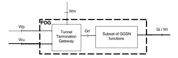
Figure 6.2.3: PDG implementation re-using GGSN functionality (from 23.234)
