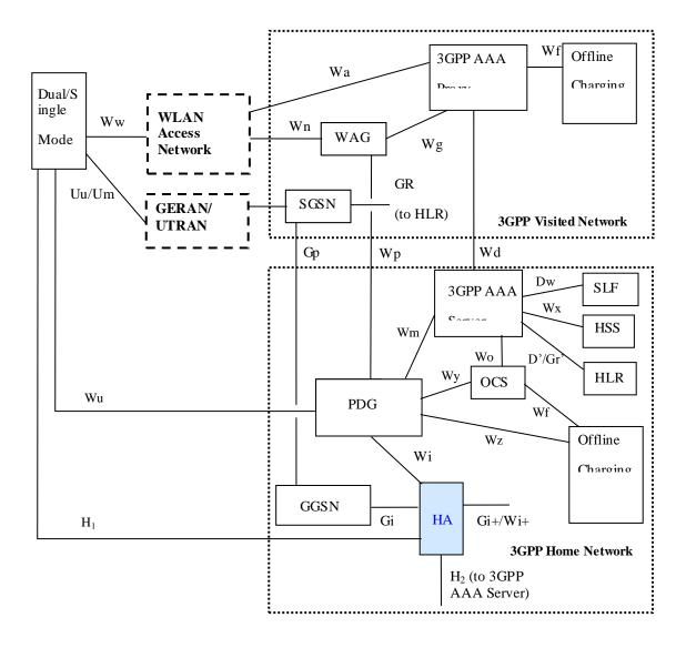
Figure 6.2.17 Alternative Roaming Architecture (with home routed traffic) for I-WLAN Mobility
