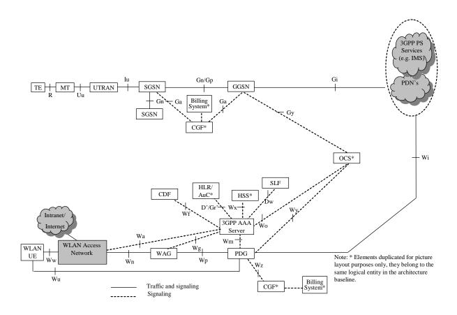
Figure 6.1.1. The baseline non-roaming architecture for defining mobility between 3 GPP PS system and I-WLAN.
