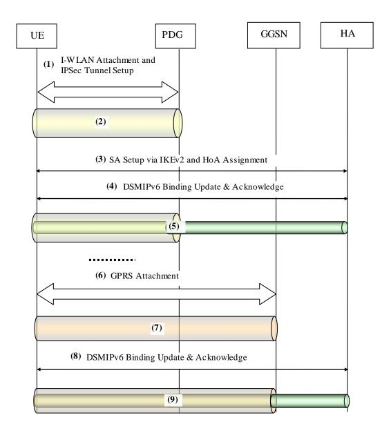
Figure 6.2.18 Information Flow for Initial Attach in I-WLAN and Subsequent Handover to GPRS (non-roaming case)
