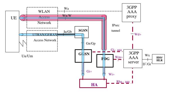
Figure A.5: Use of MIPv6 or MIPv4 with co-CoA for GPRS-WLAN mobility
