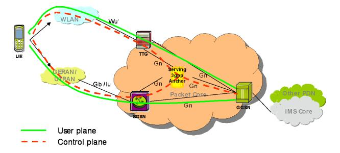
Figure 6.2.9 Handover mechanism for I-WLAN/3GPP Mobility
