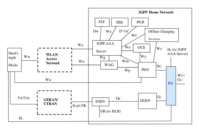
Figure 6.2.16 Alternative Non-Roaming Architecture for I-WLAN Mobility
