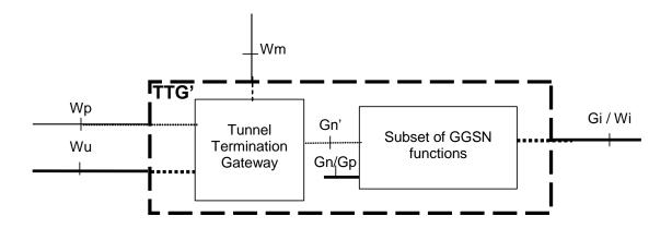
Figure 6.2.4: TTG' implementation re-using GGSN functionality
