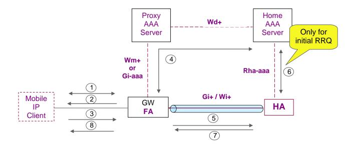
Figure A.1: Use of MIPv4 FA care-of address mode with Diameter application
