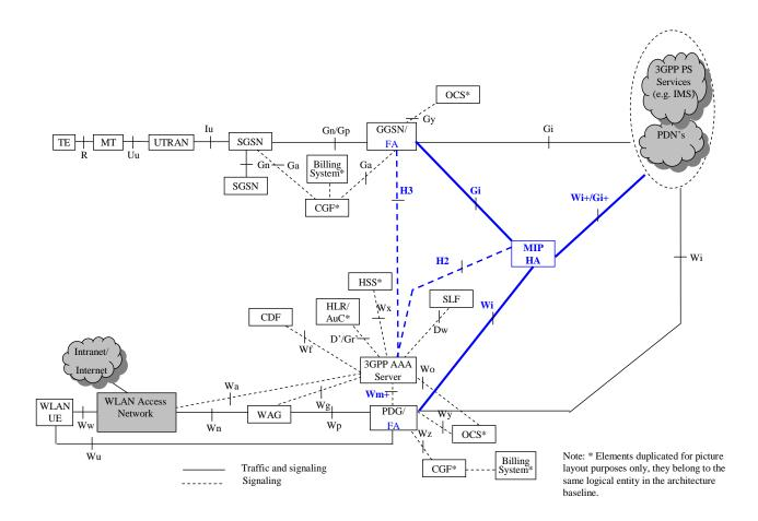
Figure 6.2.20 Solution for GPRS-IWLAN mobility based on the MIPv4 FA protocol
