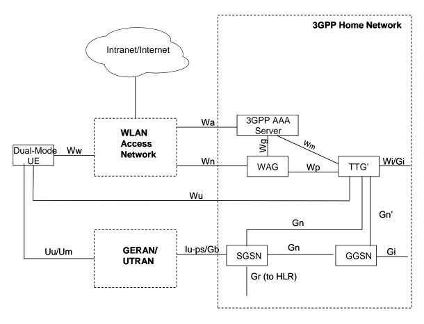
Figure 6.2.1: Non-Roaming Architecture for I-WLAN Mobility
