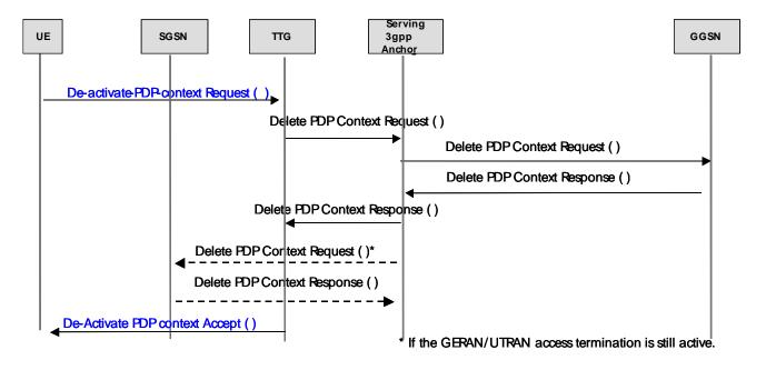
Figure 6.2.15 PDP context de-activation on the WLAN side
